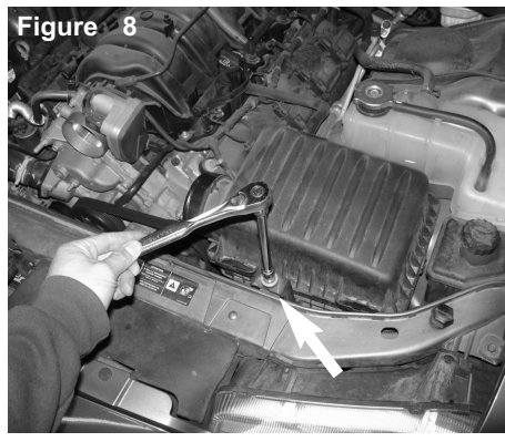
Use a 10mm socket with a 3/8 ratchet and remove the 10mm bolt mounting the factory air box to the radiator support.
