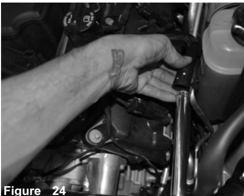
Figure 24 Connect the crank case line to the fitting on intake tube. Re-install the cover.
