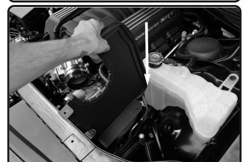
11. Now install the heatshield into the vehicle and position.
