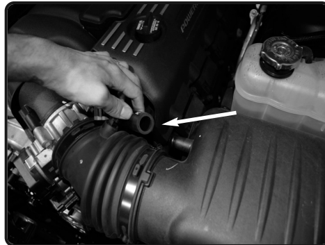
7. Pull back crank case line from airbox fitting.
