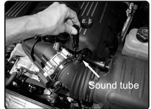
3. Loosen the clamp on throttle body using 8mm nut driver.
