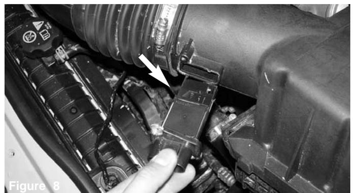
Once you have removed the screws, continue to pull the mass air flow sensor out of the sensor housing.
