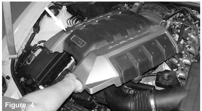
Pull the engine cover out from the stand-offs and remove the engine cover from the engine compartment.
