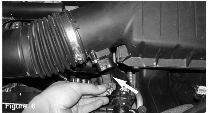
Depress the tab and pull the electrical harness connector from the mass air flow sensor.
