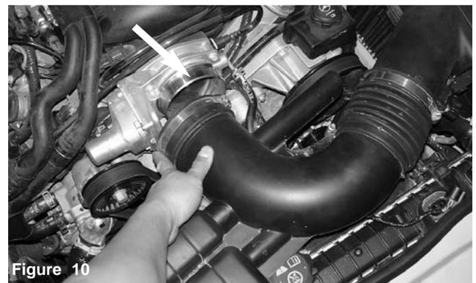
Once you have loosened the clamp, continue to pull the air intake duct from the throttle body.
