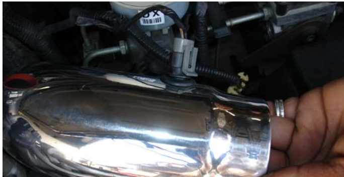
Prior to inserting the primary intake into the 3 1/2" straight hose, press the air temperature sensor into the grommet as shown above. The air temperature sensor will sit flush into the grommet.
