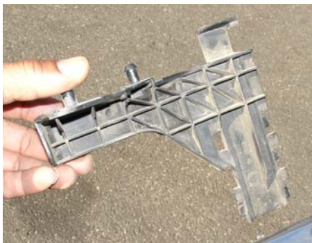
The bracket has been unhitched from the plastic pins and the bracket is now removed.
