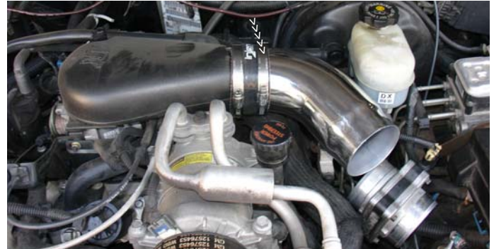
Press the primary intake into the 3 1/2" straight hose and semi-tighten the clamp at this point.
