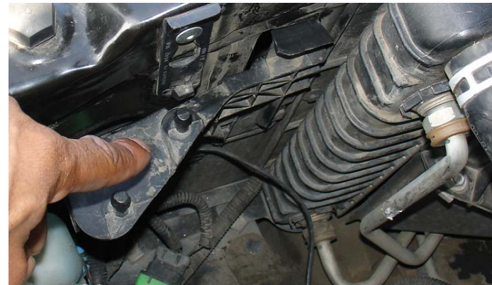
In order to make room for the new filter, the extension bracket will have to be removed.
