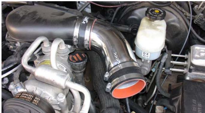
Press the 3 1/4" straight hose over the end of the primary intake and tighten the clamp that is located on the intake side.
