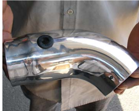
The grommet has been inserted and pressed flush into the primary intake hole.
