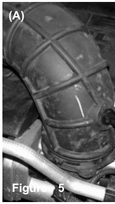
Figure 5 (A) Air temp sensor with harness removed Figure 5 (B) Firmly pull air temp sensor out of factory air duct. This sensor will be re-used later.
