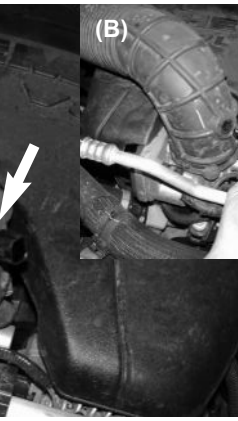
Figure 5 (A) Air temp sensor with harness removed Figure 5 (B) Firmly pull air temp sensor out of factory air duct. This sensor will be re-used later.
