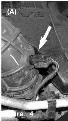
Figure 4 (A) Stock air temp sensor on factory air duct. Figure 4 (B) Unclip harness from from air temp sensor.
