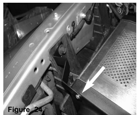
Figure 24 Loosen the bolt on the powerflow box and tighten to re-position if necessary.
