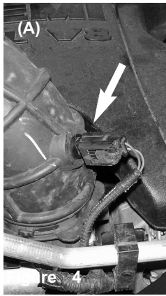
Figure 4 (A) Stock air temp sensor on factory air duct. Figure 4 (B) Unclip harness from from air temp sensor.
