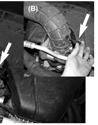
Figure 5 (A) Air temp sensor with harness removed Figure 5 (B) Firmly pull air temp sensor out of factory air duct. This sensor will be re-used later.
