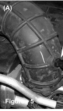
Figure 6(A) Air temp sensor with harness removed
