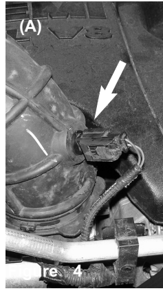
Figure 5(A) Stock air temp sensor on factory air duct.
