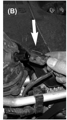
Figure 5(B) Unclip harness from from air temp sensor.
