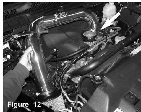
Figure 13 Position the intake pipe into the engine bay and line up the end of the pipe into the throttlebody.
