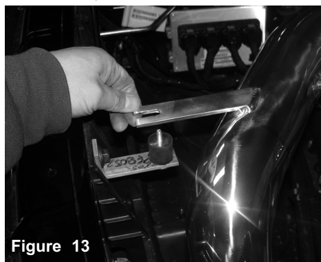
Figure 14 Align the bracket onto the vibramount
