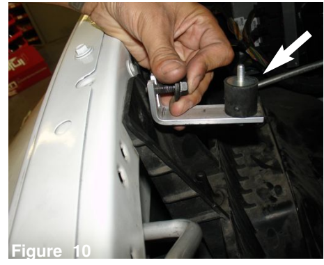
Figure 10 Loosen the front bolt holding in the air box plastic bracket closes to the headlight. Remove the bolt and save for the bracket install.
