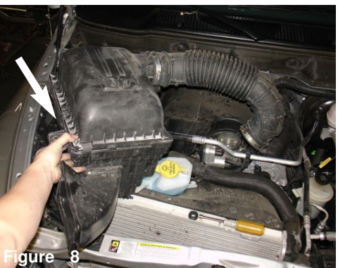
Figure 8 Disconnect the crank case ventilation tube from the factory air box cleaner. Make sure you leave the rubber coupler connected to the crank case tube.
