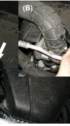
Figure 6(B) Firmly pull air temp sensor out of factory air duct. This sensor will be re-used later.
