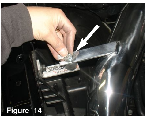
Figure 14 Align the bracket onto the vibramount.
