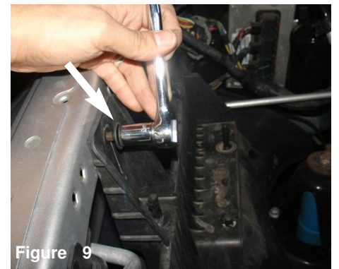
Figure 9 Lift factory air box cleaner and pull entire air box and air duct assembly out of engine bay.
