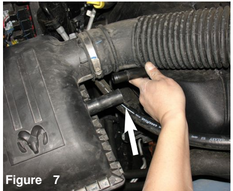
Figure 7(B) Pull air duct off of throttlebody.
