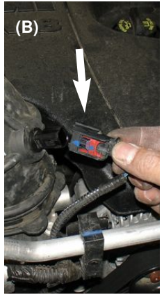
Figure 5(B) Unclip harness from air temp sensor.
