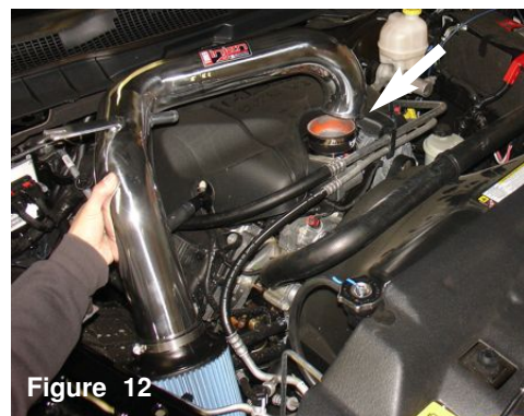
Figure 12 Place the filter onto the end of the pipe closer to the bracket.
