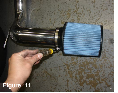
Figure 11 Install the bracket p/n: x-20091 to the spot where the bolt was removed and reuse the bolt removed from figure 8 to secure the bracket to the fender well. Install the vibramount, nut and washer to the bracket.
