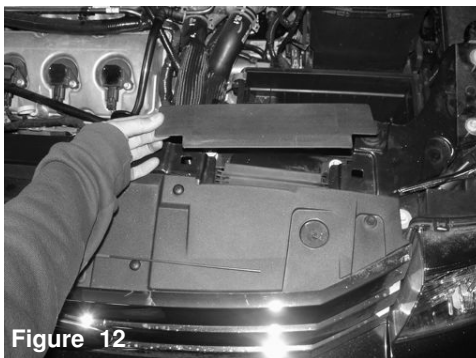
Figure 12 Lift up and remove the air scoop cover located on top of the radiator support
