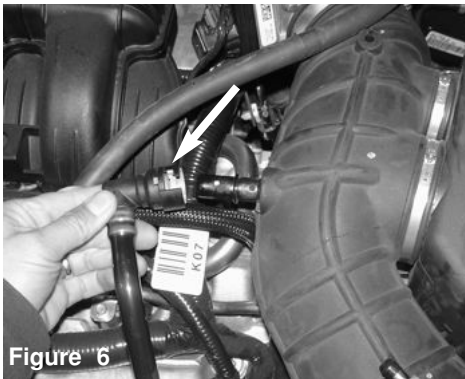
Figure 6 Pull the release tab on the left vacuum line located on the factory air duct to detach it from the fitting on the air duct
