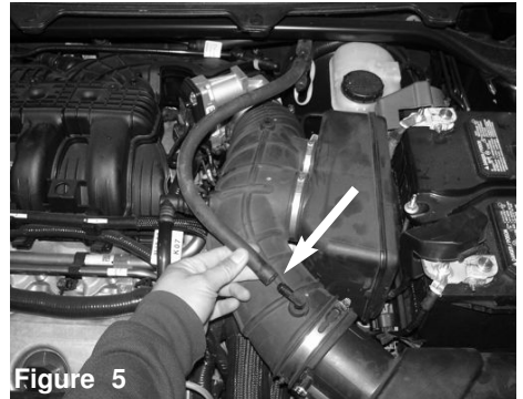
Figure 5 Detach the brake booster vacuum line from the top of the factory air duct
