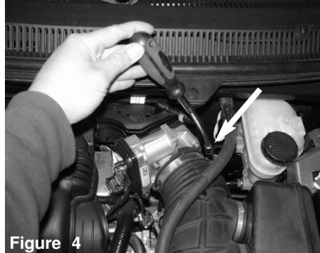
Figure 4 Use a 8mm nut driver and loosen the clamp on the factory air duct located on the throttle body
