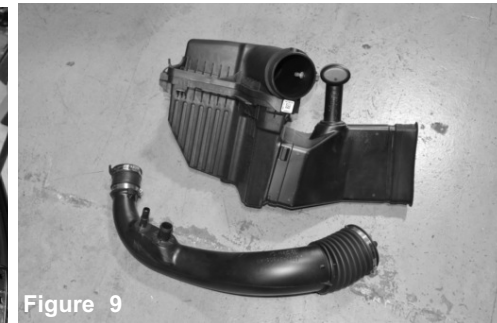
Figure 9 Shown above is the complete stock air box assembly removed.
