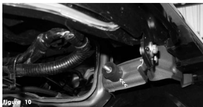
Take the male studded vibra-mount and insert it into the pre-drilled hole by the resonator opening. Screw an M6 flange nut to the vibra-mount stud under the the sheet metal.
