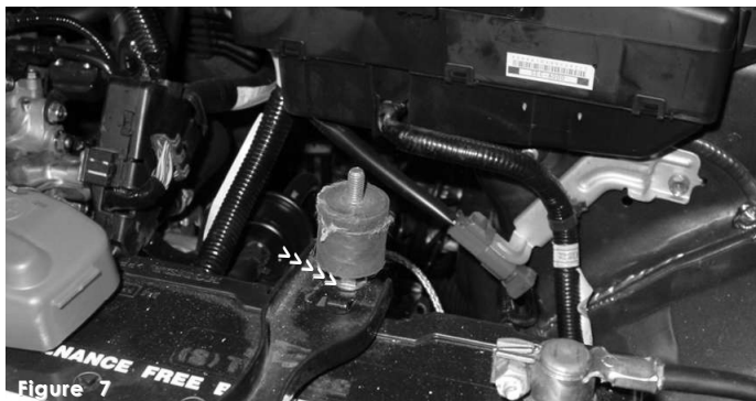
Take the male/female vibra-mount and screw it over the threaded battery post. Do not bottom out the vibra-mount a full 20 turns will be more than enough.
