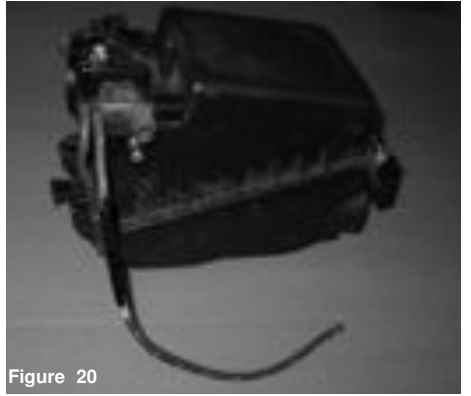
Figure 20 The assembled air box cleaner that has been removed from the engine compartment including the VAD vacuum switching valve, which is no longer used
