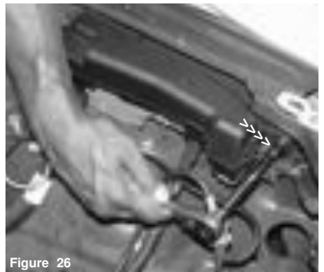
Figure 26 Loosen and remove the m6 bolt on the fuse box located on the fender wall.
