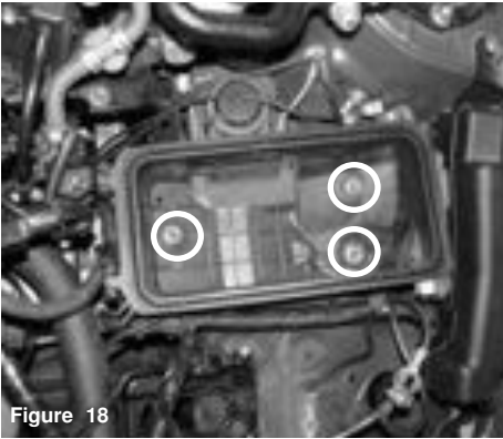
Figure 18 Once you have removed the upper air box cleaner, continue to remove the paper filter panel. Unscrew the three m6 bolts from the lower air box cleaner,
