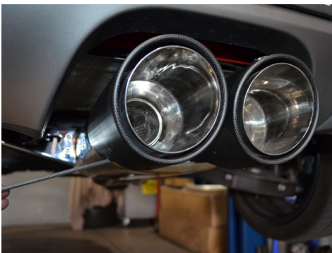
10. Adjust the exhaust tips to the desired location then secure the clamps.
