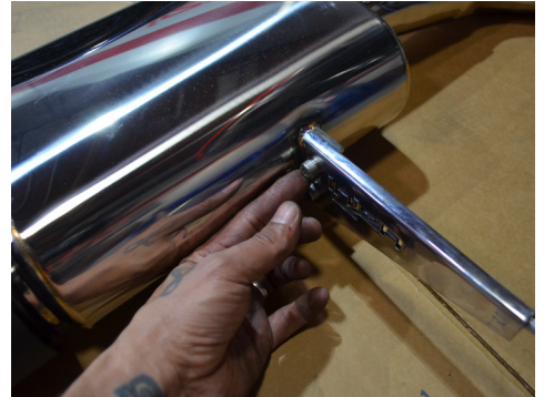
6. Secure the left and right hanger to the axle back exhaust using the provided M8 x12mm bolts
