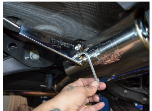
9. If needed, readjust both hanger brackets.
