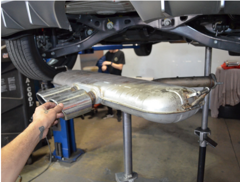
4. Remove the OEM muffler section from the vehicle.
