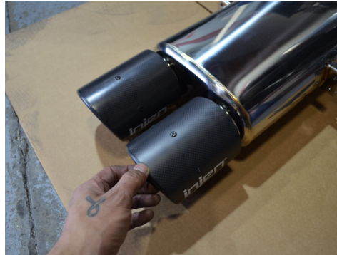
5. Attach the provided tips to the Injen axle back exhaust. Do not fully secure until the exhaust is mounted on the vehicle.
