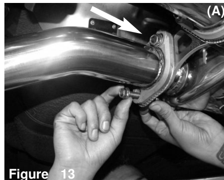
Figure 13 Secure the two parts using provided M10 bolts and nuts. DO NOT TIGHTEN!
