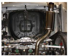
The new SES1898TT is finally here. A full 76mm slip-fit straight through, featuring a Titanium tip with an embossed Injen logo. This system when used with the test pipe already included in this kit delivers up to 25 h/p to the wheels. The street version exhaust system comes with a S.S. tip and flanges for ease of installation (SES1898).
