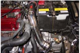
Insert the primary intake into the 90 degree hose on the throttle body, use two .312 Power-bands (A). Align the hardpiping and semi-tighten the clamps. Press the 2 1/2" straight hose over the end of the pipe and use two .312 Power-Bands (B). Tighten the clamp on hardpipe (A).
