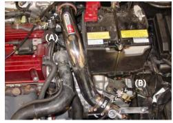
Hardpipe (B) connects to the driver side end tank outlet and to the upper hard pipe (A). The stock elbow is used on both sides of the tank.
