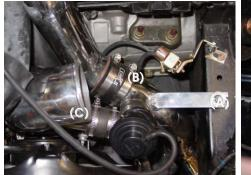
Top view of the bracket (A), blow-off valve (B) and cast intake (C) all connected and ready for the next step.
