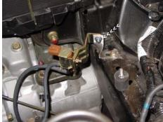
Mount the boost control solenoid bracket to the 1450T bracket. Use an m6 x m16 hex bolt and flange nut.
