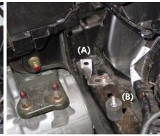
Take the small 1450T bracket and mount it to the held the air intake box and boost solenoid in place. frame of the car, use the stock bolt to secure the bracket in place(A). Screw the vibra-mount into the pre-tapped hole on the same frame as the bracket(B).
