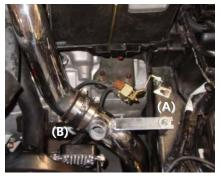
The secondary hardpipe bracket will align to the vibra-mount stud(A). Use the m6 nut and washer to hold the intake in place. Insert to top end into the 2 1/2" hose and align the intake before you semi-tighten any of the clamps(B).
