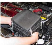
The stock air intake box is removed and the mass air flow sensor is disconnected from the air intake box to be used later in the instruction.
