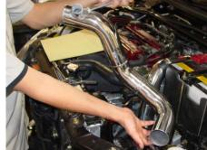
Take the secondary hardpipe and lower it into the bumper section. Insert the lower end into the stock hose on the intercooler port but do not tighten the two .312 Power-bands that are to be used.
