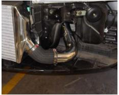
Here is a shot of hardpipe (B) connected to the stock hose on the intercooler tanks. Use two .362 Powerbands to connect hardpipe (B) to intercooler end tank.
