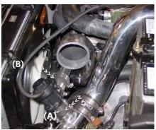
Insert the assembled blow-off valve over the large port on the intercooler pipe(B). Press the other end over the large port on the intake(B). If another manufacturers intake is being used some modification will be required.
