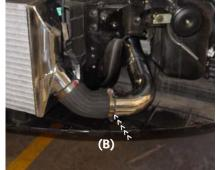
Hardpipe (C) connected to passenger side intercooler end tank inlet. The side seen here is the hardpipe connected to the turbo outlet.
