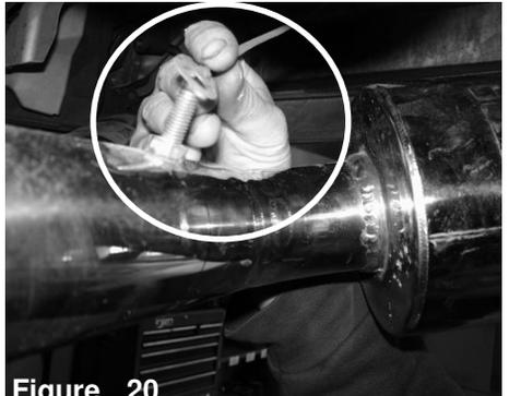
Connect the grounding wire located at the rear of the vehicle to the welded bolt on the driverside muffler piping.
