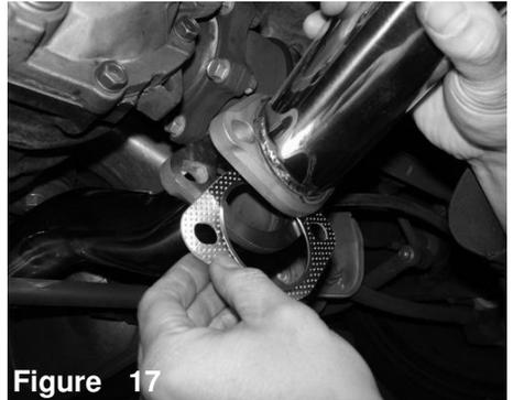
Place a 60mm gasket in between the rear muffler and mid-pipe on both left and right side.
