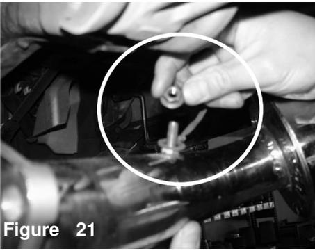
Place a supplied M8 nut to the welded bolt and secure the grounding wire to the Injen exhaust system.
