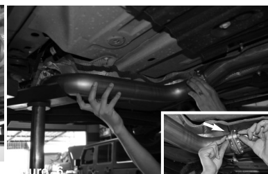
Figure 6 Once the mid-pipe is in place. Use provided 76mm gasket and 2 bolts and nuts. Do not tighten.
