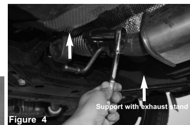
Figure 4 Loosen the 2 15mm nuts on OEM downpipe flange using ratchet and socket. Save nuts and gasket for later use. Remove the factory front section.
