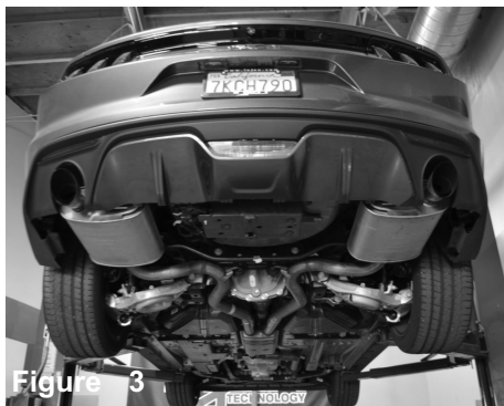
Figure 3 OEM exhaust system. Secure vehicle on lift.
