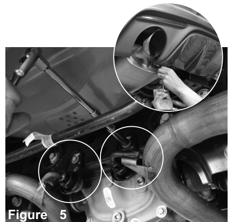
Figure 5 For easier removal, loosen the 13mm bolts holding in the exhaust rubber isolation mounts. Remove the rear muffler isolation mounts also using 13mm socket and ratchet.
