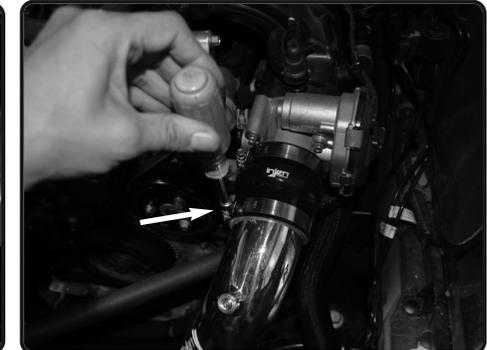
**7.** Tighten all clamps using 8mm nut driver.
