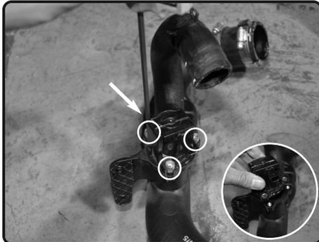
**12.** Loosen the 3 screws holding in the diverter valve using allen key. Carefully remove. Position new injen intercooler next to pipe for correct position.
