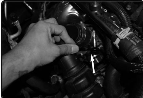
**8.** Loosen the clamp on the turbo for the hot side of the intercooler pipe using 7mm nut driver or ratchet. Loosen the clamp on the intercooler side also.
