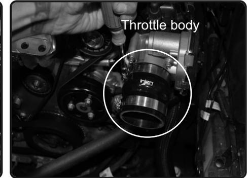
**3.** Install the provided 2-3/4" hump hose to the throttle body using provided clamps, tighten the clamp on throttle body only.
