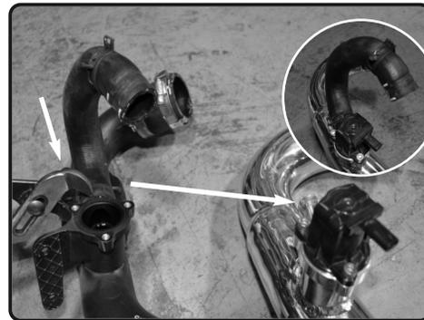
**14.** With pliers loosen, loosen clamp and pull back line. Carefully remove and transfer to the new injen intercooler fitting.
