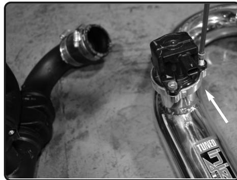
**13.** Secure the diverter valve to the injen intercooler pipe using allen key. Secure using original screws.
