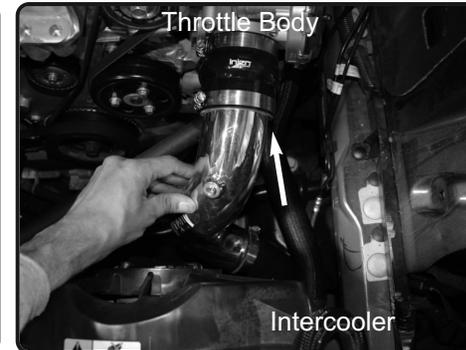
**6.** Now position the intercooler pipe into the hump hose on throttle body and secure. Adjust for proper fitment.
