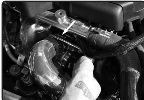
**21.** Secure the turbo side of the coupler and tighten using 8mm nut driver.
