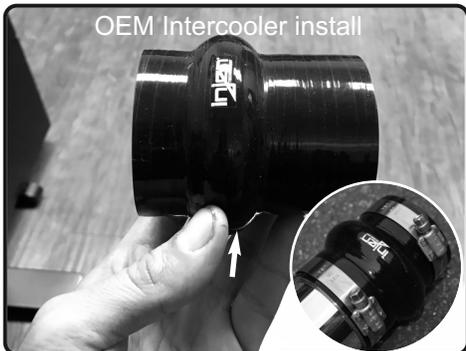
**16.** The 2.5" x 3.5"L hump hose seen above is for the installation with OEM intercooler only! **DO NOT CUT!**
