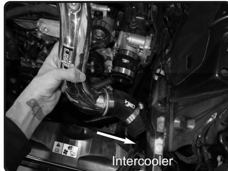
**5.** With soap water lubrication on the inside of the elbow hose, install the intercooler assembly into vehicle with clamp. This will allow for the elbow hose to slide on easier to intercooler. Do not tighten.
