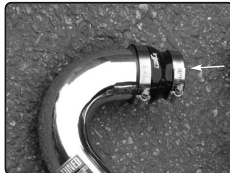
**18.** Install the step hose with clamps provided to the turbo side of the intercooler pipe.
