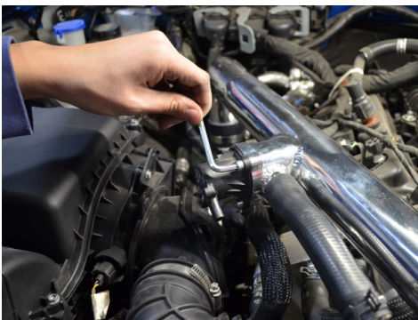
46. Reinstall the diverter valve to the Injen tube. Secure using the provided M6 socket head bolts.
