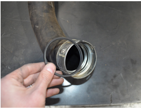
25. Remove the OEM O-ring from both intercooler hoses. Note the direction it was removed in.
