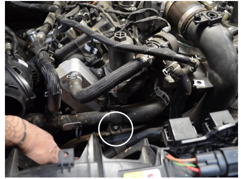
15. Remove the bolt securing the cold side intercooler pipe to the bracket.
