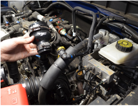
49. Attach the 1.50"-2.25" stepping hump hose to the driver side turbo outlet. Secure using the provided clamps.
