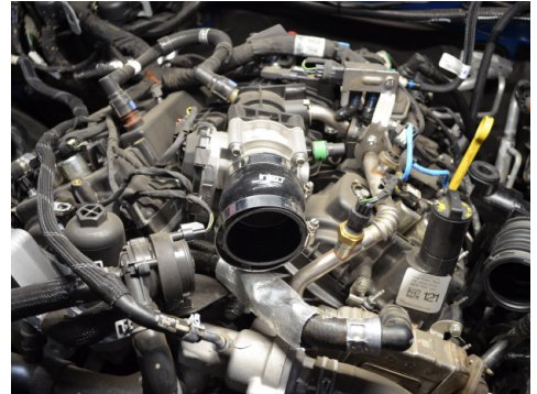
30. Attach the 2.75" hump hose to the throttle body. Secure using the provided clamps.
