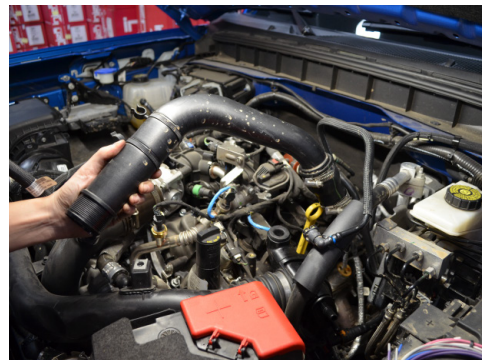
9. Remove the driver side intercooler pipe.
