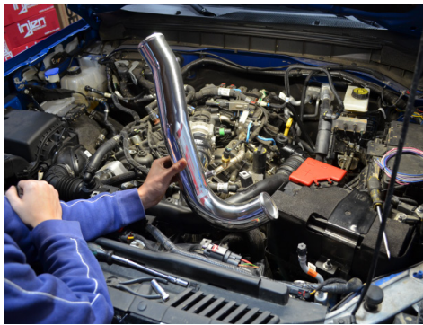
38. Install the primary hot side intercooler pipe.
