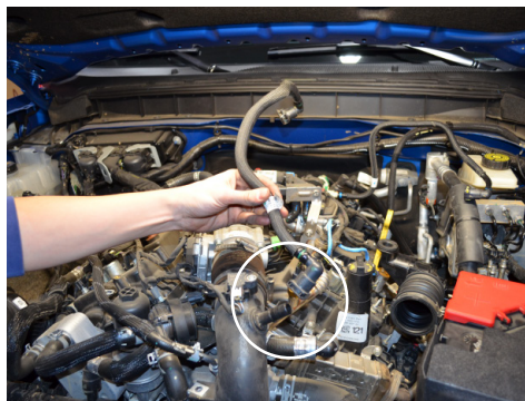
11. Disconnect the crankcase line on the cold side intercooler pipe by pressing down on the locking clip.
