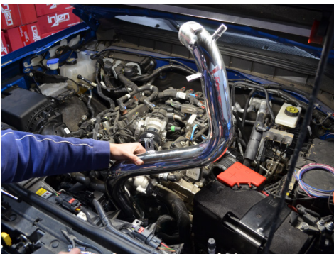
31. Install the Injen cold side intercooler pipe. Secure to the vibra-mount once the pipe is in place.
