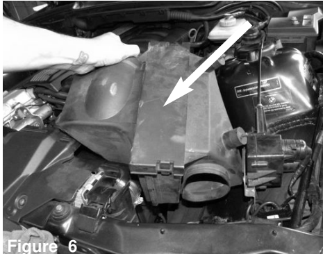
Figure 6 Carefully lift up and pull out the air box.
