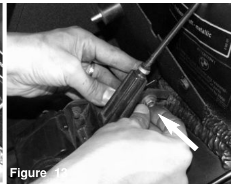
Figure 10 Attach the other vibra mount to the tab on housing. Secure using provided nut and washer. Tighten using 10mm socket and ratchet.
