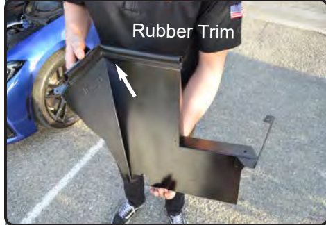
9. Install the provided Rubber trim to the top of the heatshield. Notch corner with pliers/cutters for easier installation.
