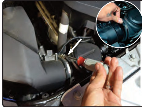
3. Loosen the clamp on the air box using 6mm nut driver. Pull back the intake tube from the air box.
