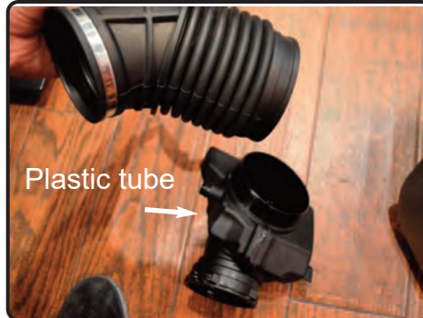
7. Remove the intake tube from the hard plastic intake tube. Make sure the Lock clip is seated correctly in the intake tube to allow the tube to secured properly to turbo.
