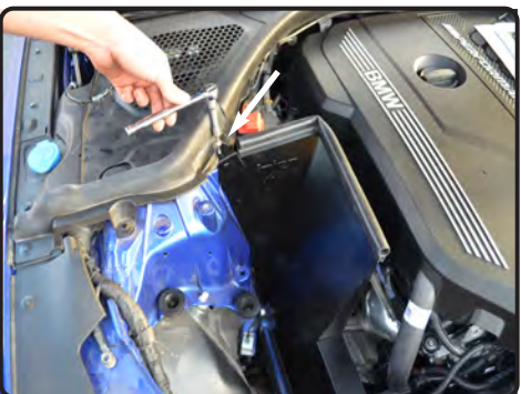
16. Secure the tab on heatshield using the OEM torx screw. Secure and tighten.
