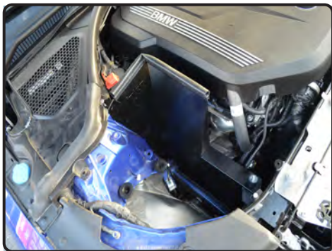
17. Complete heatshield assembly installed. Tighten all screws and secure.
