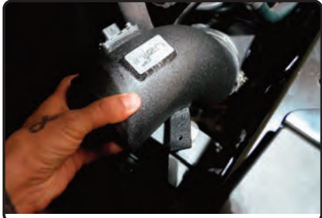
21. Install the intake tube into the vehicle and position to the straight hose and bracket to the vibramount.
