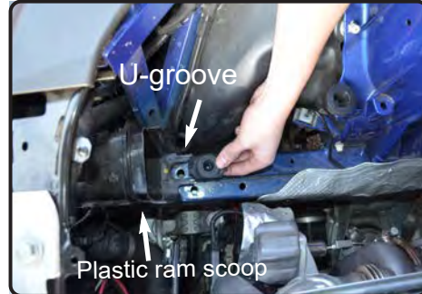
11. Remove the Air box grommet located on the frame in front of Plastic ram scoop. Heat shield will seat inside this plastic U-groove.
