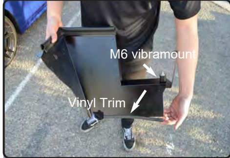
10. Install the provided Vinyl trim to the bottom of the heatshield. Install the M6 vibramount to the Threaded insert on heatshield.
