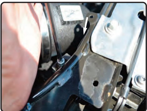
15. Secure the heatshield tab to the radiator support using M6 screw and M6 nut. Secure and tighten allen key.
