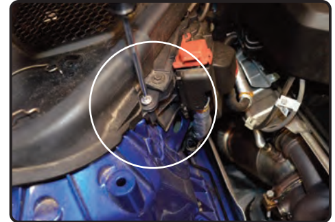
12. Loosen the T30 torx screw located near Positive battery terminal. Save bolt for later install.
