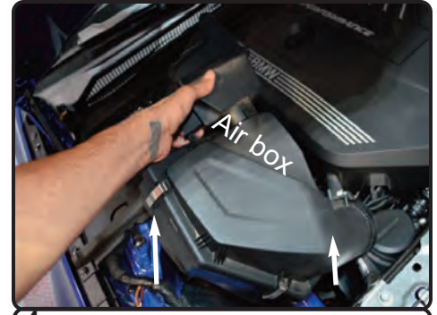
4. Carefully lift up and remove the airbox from the vehicle. Note: Next photo intake tube was removed for easier look at intake tube and for photos.
