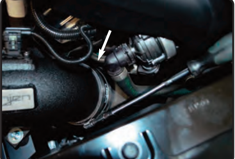
23. Tighten the clamp on the intake tube using 8mm nut driver.
