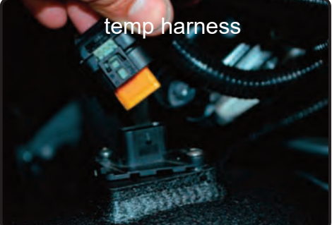
24. Re-connect the temp harness.
