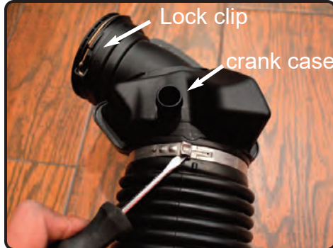
5. With a flat head screw driver, pull back the lock clip on the turbo. Slide out intake tube from turbo. Disconnect the crank case line on the intake tube by depressing clip. With flat head screwdriver, break the security clamp loose.
