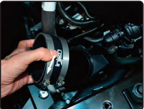
20. Install the provided 4" straight hose with clamps to the plastic intake tube. Tighten clamp on the plastic tube only.
