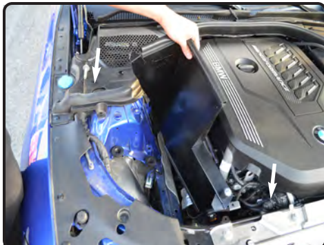
13. Install the heatshield into vehicle. Front tab will fit under the radiator support.
