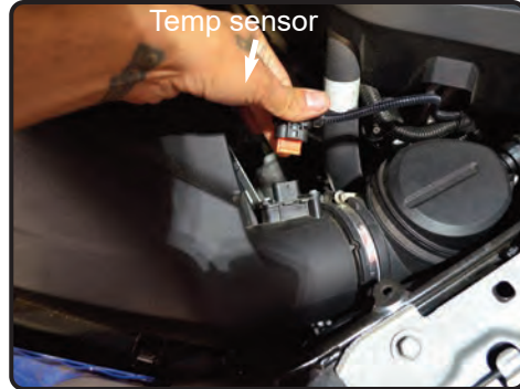
2. Disconnect the Temp sensor harness and pull harness cable from the air box.
