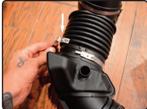
6. Remove the security clamp from intake tube.
