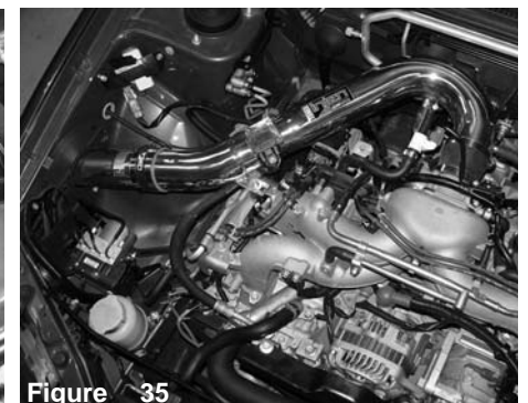
Figure 35 Align the entire intake for the best possible fit. Once you have cleared the intake from all moving parts, continue to tighten all nuts, bolts and clamps.
