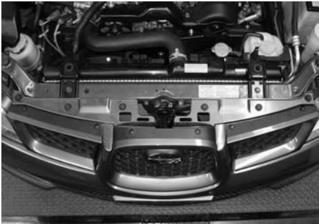
Figure 2 Removal of front bumper is required. Remove the 6 big plastic clips, 4 small clips on grill on top. Remove both front grills.
