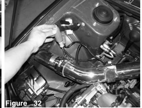
Figure 32 Tighten all clamps on silicon elbow hose in both images using 8mm nut driver. Once you have aligned and tightened all nuts, bolts and clamps, continue to install the front bumper to its original position.
