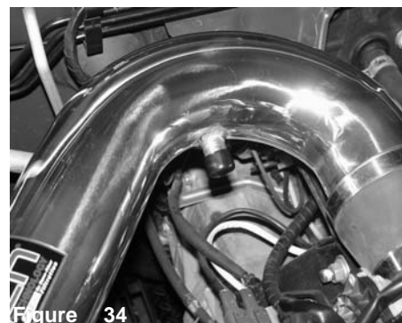
Figure 34 2005 model only cap off the 5/8 fitting.
