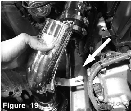
Figure 16 Install the intake tube and position the tube to the hose on the throttle body.
