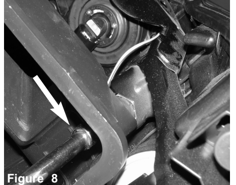
Figure 8 If vehicle is equipped with front bolt, remove the 10mm bolt using 10mm socket or wrench.
