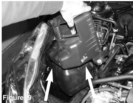
Figure 9 Loosen the 2 10mm bolts holding in the OEM air box and remove.
