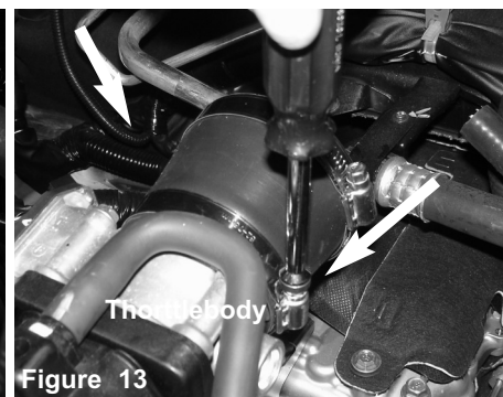
Figure 13 Install the provided step hose with clamps provided to the throttle body.
