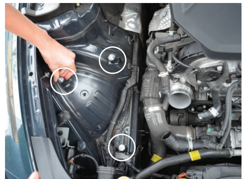
12. Secure the provided vibra mounts to the the threaded holes on the chassis. The bottom vibra mount will mount onto the threaded stud.
