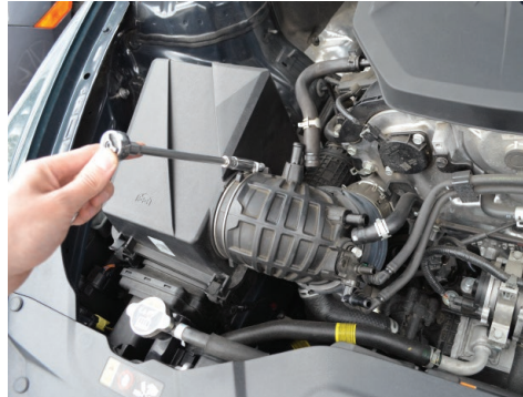
5. Loosen the clamp securing the intake tube to the airbox.
