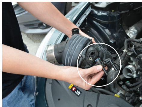
11. Detach the evap fitting from the intake tube. This fitting will be reused on the injen intake. Ensure the O-Ring stays on the fitting.
