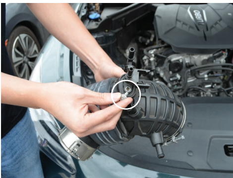
10. Remove the bolt securing the evap fitting.
