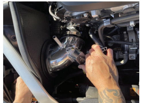
21. Install the injen intake tube, then secure with the provided clamp.
