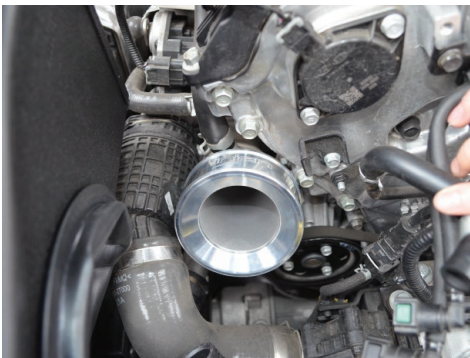
19. Attach the turbo inlet adapter to the turbo. You should hear the C-Clip engage once secure.
