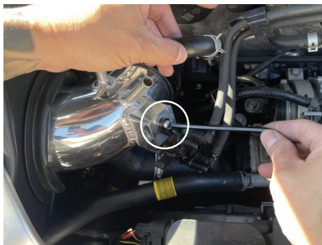
23. Secure the evap fitting with the provided M6 bolt.
