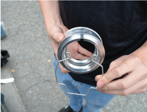
16. Install the C-Clip onto the injen turbo inlet adapter
