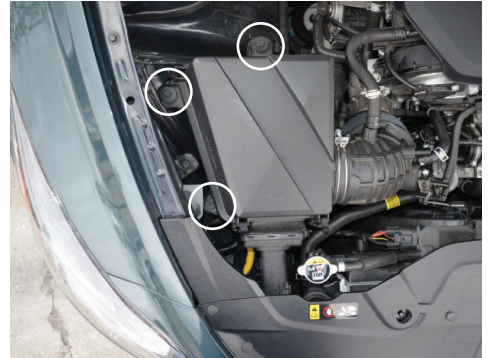
6. Remove the three bolts securing the airbox to the engine bay.
