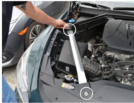
2. Remove the two bolts securing the passenger side strut brace, then remove the strut brace.
