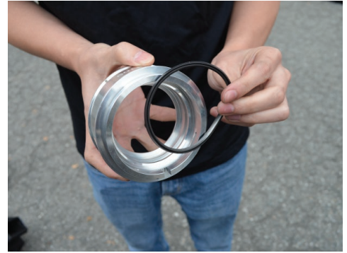
18. Install the O-Ring onto the turbo inlet adapter in the same direction it was removed.
