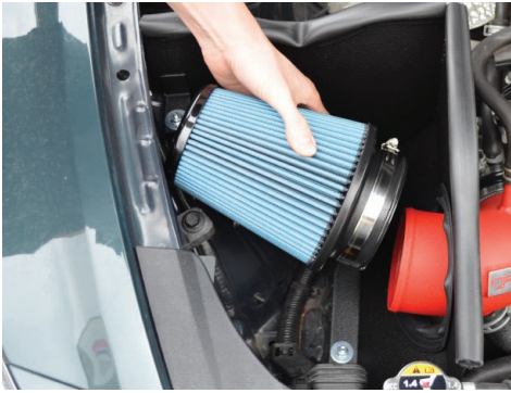
25. Install the air filter to the intake tube and secure using the provided clamp.
