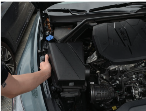
7. Detach the intake tube from the airbox, then remove the airbox from the engine bay.
