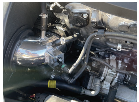
24. Secure the three crank case lines to the intake tube with the oem tension clamps. Reattach the evap lines to the evap fitting.
