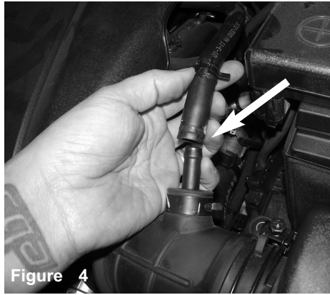
Now with pliers, loosen the clamp holding in crank case line and pull back.
