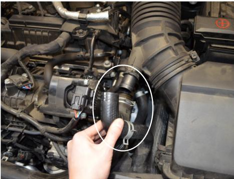
4. Disconnect the diverter valve hose.
