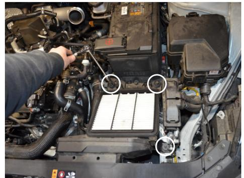
9. Remove the three bolts securing the airbox.
