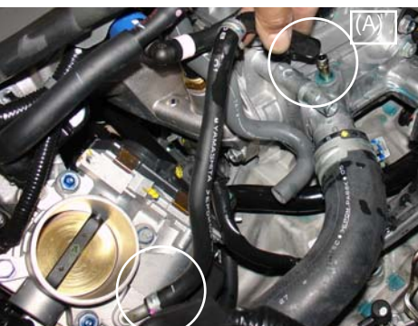
Referring to top middle picture or figure A, the (C) is disconnected from the PCV hard pipe and pressed over the coolant outlet port (A).
