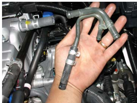
PCV hard pipe has been disconnected and removed from the breather hose and coolant lines.
