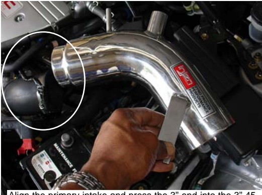
Align the primary intake and press the 3" end into the 3° 45 degree elbow.
