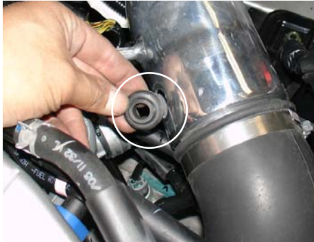
Insert the 1525 sensor grommet into the pre-drilled 3/4" hole. The grommet groove will sit flush in the 3/4" hole inner diameter.
