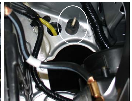
Screw the male m6 vibra-mount into the pre-tapped hole right above the resonator opening.
