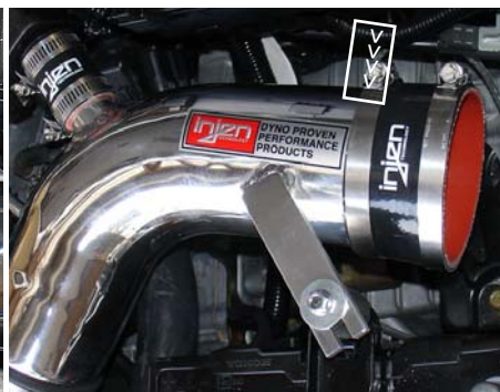
The 3 1/2" straight hose is pressed over the end of the primary intake. Use two large clamps and tighten the clamp on the intake side
