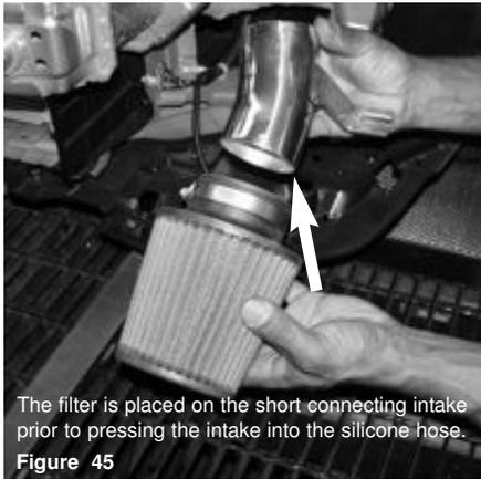
The filter is placed on the short connecting intake prior to pressing the intake into the silicone hose.
