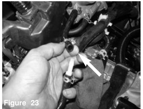
Figure 20 Loosen the clips on the hard line and slide back. This will be removed and secured with a 1/4" vinyl coupler. Note: Place a shop rag under neath and make sure vehicle is cold and not warm, there will be some coolant leaking.
