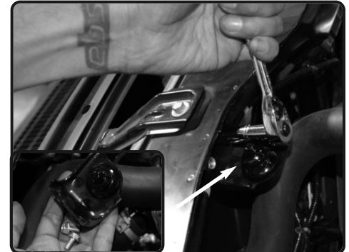
7. Loosen the OEM air box bracket out of vehicle using 10mm socket or wrench. Save 1 screw for later install.
