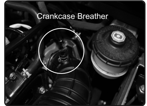
3. With pliers, remove the hard crankcase line out of the intake tube.
