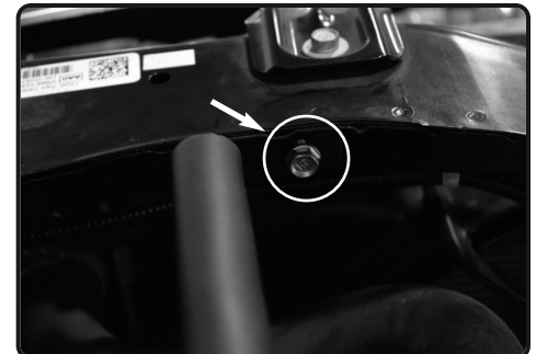
11. Now secure the back bracket to the factory air box mounting position. Secure using OEM screw from step 7.
