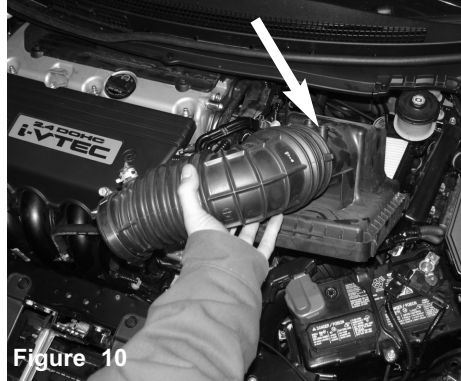
Figure 10 Now pull the upper air box assembly forward and out.
