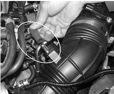
The air control thermal vacuum hose is disconnected from the air intake duct.
