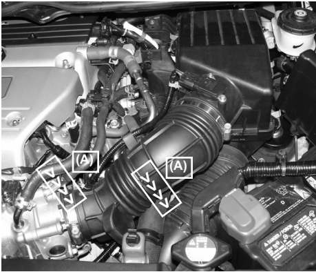
Stock air intake box ready to be removed from the engine compartment. Start by loosening the clamps at the air resonator duct (A) and throttle body (B).
