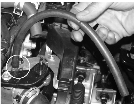
Press the 12"-6mm vacuum line over the upper coolant outlet port. Use the stock clamp to secure the vacuum hose in place.
