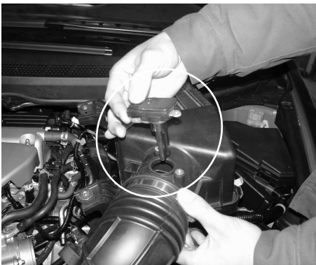
Remove the two screws holding the mass air flow sensor to the air intake box as shown above.
