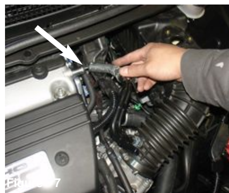
Figure 4 Figure A: Disconnect the MAF sensor harness. Figure B: Use a phillips screw driver and remove the two screws on the MAF sensor.
