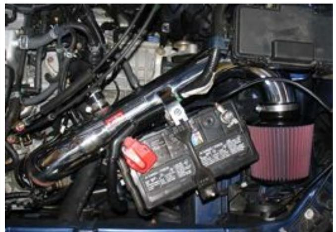
**Prior to starting this installation, disconnect the negative battery terminal.**
