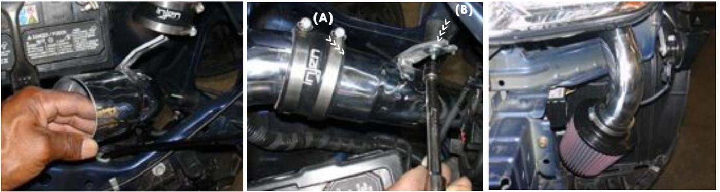
Locate the secondary intake and insert it into the bumper area via the engine compartment between the battery and front cross member.
