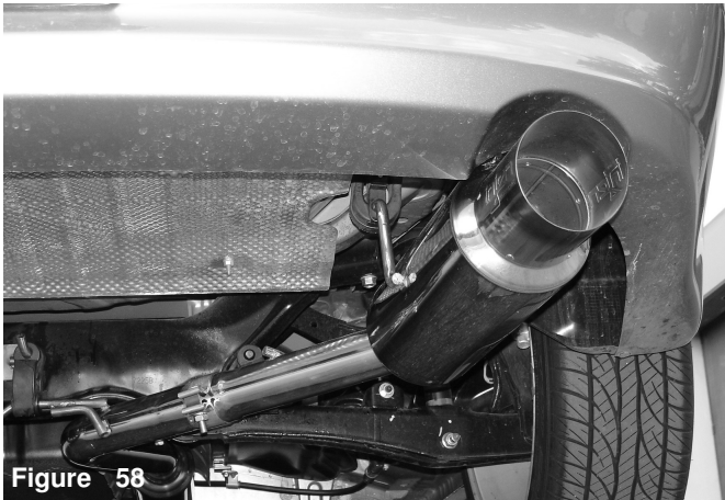
Figure 58 Driver under shot of the bolt-on exhaust system for easy installation.
