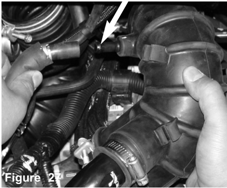
Figure 27 Once you have removed the tension clamp from the intake vacuum port, continue to pull the CC hose from the air intake port.
