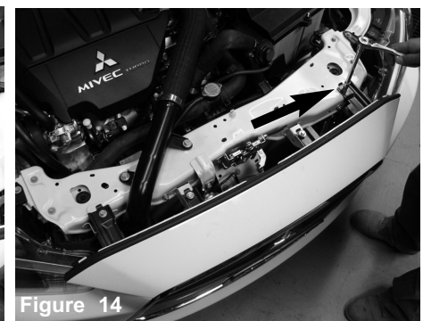
Figure 14 The first 10mm bolt is loosened and removed. There are an additional 5-10mm bolts and 4 clips underneath the bumper that need to be removed prior to pulling the bumper off.
