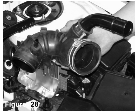
Figure 28 The air intake duct is now ready to be pulled out of the engine compartment.
