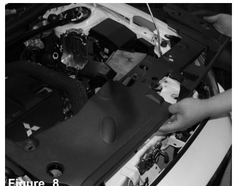
Figure 8 Once all three plastic clips have been removed, continue to pull the shroud from the engine compartment.
