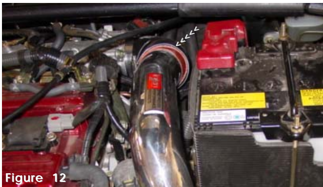
Figure 12 Insert the primary intake into the 90 degree throttlebody elbow, and use two clamps. Align the intake and semi-tighten the clamps.
