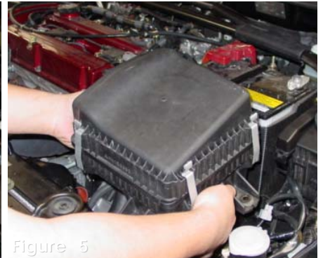
Figure 5 The stock air intake box is removed and the mass air flow sensor is disconnected from the air intake box to be used later in the instruction.
