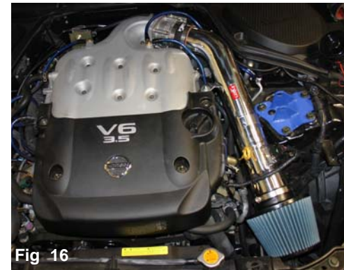
Fig 16 The cold air intake is seen in this picture used as a short ram.
