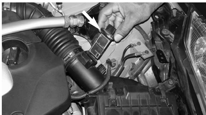
Figure 7 Loosen the air duct clamp that connects the air duct to the sensor housing.
