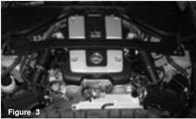
Figure 3 Stock air intake cleaner and air ducts shown in this picture. Before getting started with the installation, disconnect the negative battery terminal.
