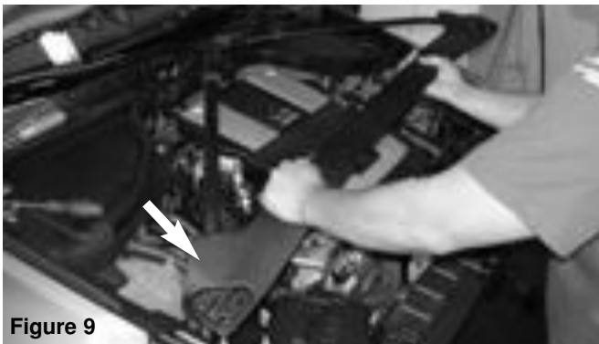
Figure 9 Once you have removed all nuts and bolts, continue to pull the stabilizer bar out of the engine compartment.
