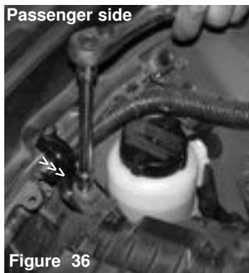
Use a 10mm socket to loosen the bolt securing the air box cleaner in place. There is one bolt on the the passenger and driver side.
