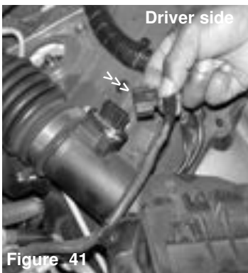
Depress the plastic tab and pull the harness clip from the mass air flow sensor.
