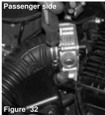
Loosen the clamp on both the passenger and driver side throttle body air intake ducts.
