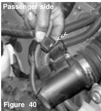
Depress the plastic tab and pull the harness clip from the mass air flow sensor.
