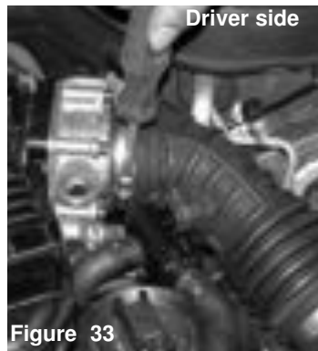
Loosen the clamp on both the passenger and driver side throttle body air intake ducts.
