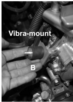
A) Locate the passenger side bracket on the engine. B) Install provided M6 vibramount with nut to the bracket. Center the bracket to the slotted hole and tighten using 10mm wrench.
