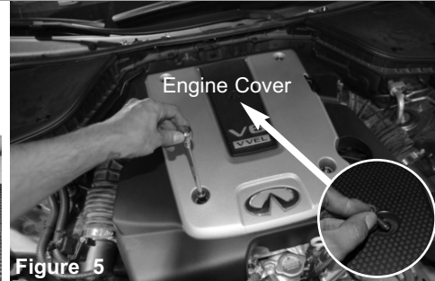
Figure 5: Remove the 3 bolts and 2 nuts holding in the engine cover. Lift up and remove the engine cover.
