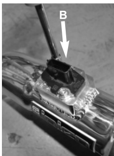
A) For both passenger and driver install the straight hose with clamps provided to the throttle body's. B) Install the filters to the intake tubes and tighten using 8mm.
