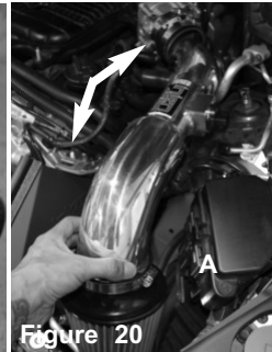
1. Upon completion of the installation, reconnect the negative battery terminal before you start the engine. 2. Align the entire intake system for the best possible fit. Once the intake has been properly fitted continue to tighten all nuts, bolts and clamps. 3. Periodically, recheck the alignment of the intake system and make sure there is proper clearance around and along the length of the intake. Failure to follow proper maintenance procedures may cause damage to the intake and will void the warranty. 4. Start the engine and listen carefully for any odd noises, rattles and/or air leaks prior to taking it for a test drive. If any problems arise go back and check the vacuum lines, hoses and clamps that maybe causing leaks or rattles and correct the problem. 5. Check the filter for excessive dirt build up. Clean or replace the filter with an original Injen filter (can be bought on-line at "injenonline.com"). Congratulations! You have just completed the installation of the best intake system sold on the market. Enjoy the added power and performance of your new intake system.
