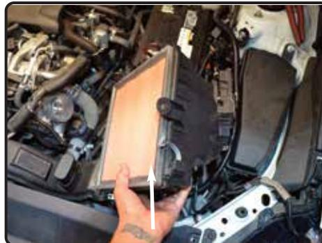
7. Lift up and remove the lower part of air box out of vehicle. Leave the front OEM ram scoop in vehicle.
