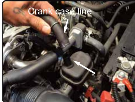
3. Push the factory clamp in and pull back the crank case line away from the intake tube.
