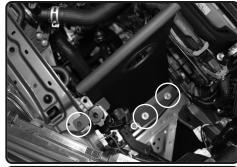
**11.** Install the heatshield to the vehicle. Use the screws from step 5 to secure heatshield. Re install the screw from step 9 to the bracket and secure and tighten.
