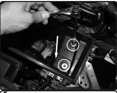
**5.** Loosen the 2 bolts holding in the lower part of the air box. Remove the bottom half of the air box out of vehicle.
