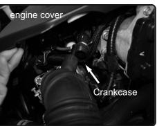
**2.** Pull back the engine cover. Remove the crankcase line from the stock intake tube.
