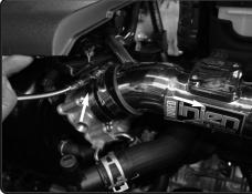
**15.** Now install the step hose to the throttle body. Tighten clamp on the throttle body only using 8mm nut driver.
