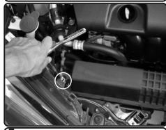
**7.** Loosen the 2 bolts holding in the OEM air box ram scoop and remove.
