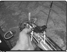
**13.** Now install the MAF sensor into the new injen tube. Secure and tighten using provided M4 screws.
