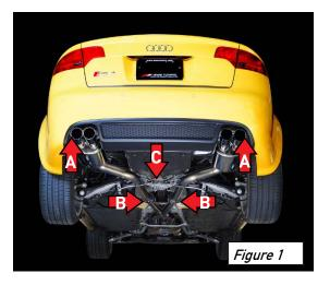
Each rear tip is rotationally adjustable to ensure that the AWE Tuning logo remains centered when the exhaust is installed, and also length is adjustable to suit personal taste.
