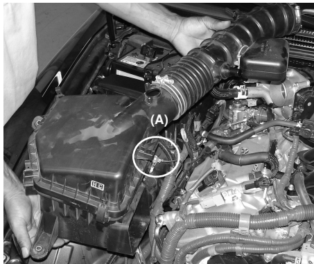
Lift and Pull the air box cleaner from the lower grommets. Before pulling the air box out, unclip sensor harness from the air box side clip (A).
