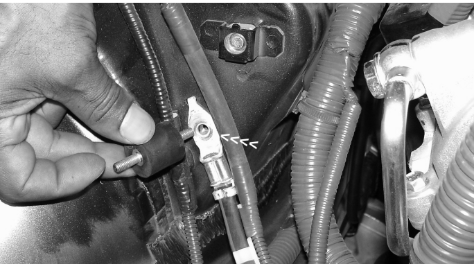
Once the screw has been removed, continue to place the vibra-mount into the pre-tapped hole as shown above.
