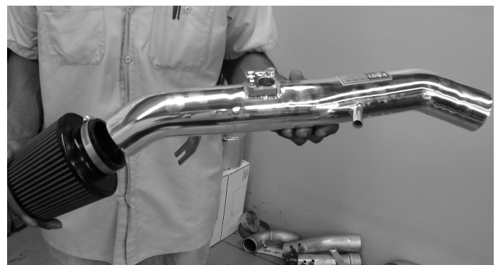
Slip the three inch filter over the end of the intake until it butts up against the filter stops. Once the filter has been firmly placed, continue to tighten the filter neck clamp.
