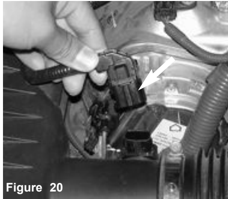
Depress the tab and pull the electrical harness connector from the mass air flow sensor.
