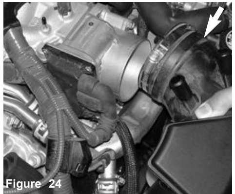
Once you have loosened the clamp, continue to pull the air intake duct from the throttle body.
