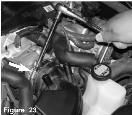
Loosen the throttle body clamp over the air intake duct.
