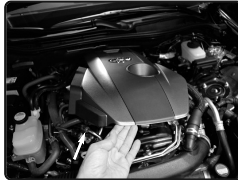
2. Lift up and remove the engine cover.
