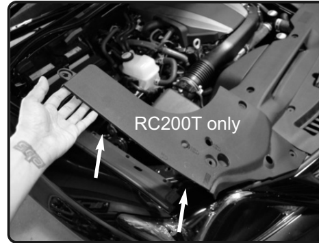
7. RC200T remove the plastic push clips, remove the side engine cover.
