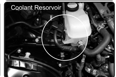
11. Locate the coolant reservoir screw, loosen this bolt and save for later install.
