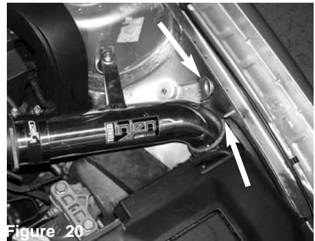
Figure 20 NOTE: Be careful with these two component in the engine bay when install the intake tube. Coming in contact with these can scratch the finish on the intake tube!
