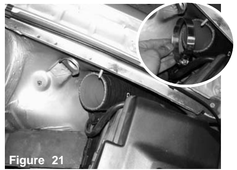
Figure 18 Mount the vibramount on to the factory bracket already mounted on the drivers side shock tower. Vibramount shown mounted on shocktower.
