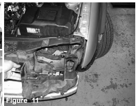
Figure 8 Figure A: There are 11 T20 torx bolts on the bottom side of the bumper that will need to be removed in order to remove the front bumper. Figure B: You may now remove the front bumper by pulling forward.
