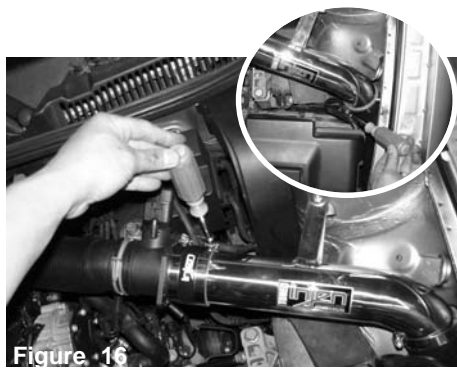
Figure 16 Once you have made final adjustments for the best fitment, use a 8mm nut driver and tighten the clamp on the MAF sensor hose and also the clamp on the TT silicon hose.
