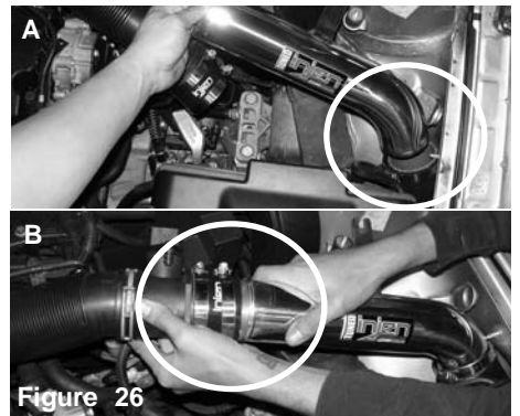
Figure 23 Place the smaller aluminum intake tube into the silicone hose and make sure you add a 040 clamp onto the silicone intake tube.
